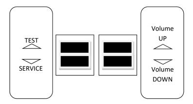
TEST button enters diagnostic system. **IMPORTANT NOTE: You must hold down the TEST button** for a least 2 seconds to Enter the Test Menu.
